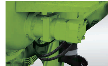
双唇密封新型搅拌结构 New Mixing Structure with the Double Lip Seal
